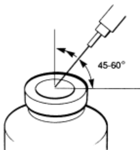
Figure 2: Method to minimize coring.
