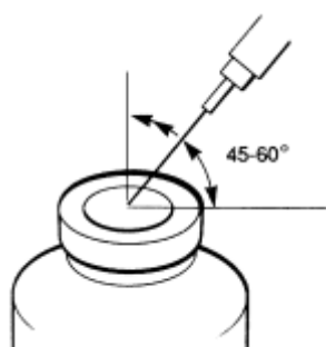
Figure 2: Method to minimize coring.
